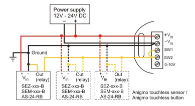
Any touchless sensor or button with relay or OC output can be used to control a DMS-CG series universal dimmer.
