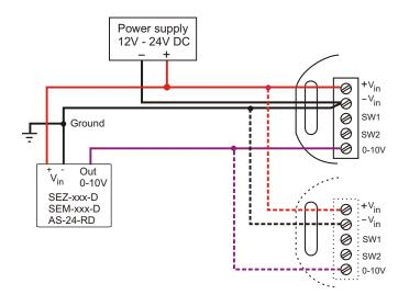
Any touchless sensor or button with 0-10V output can be used to control a DMS-CG series universal dimmer.
